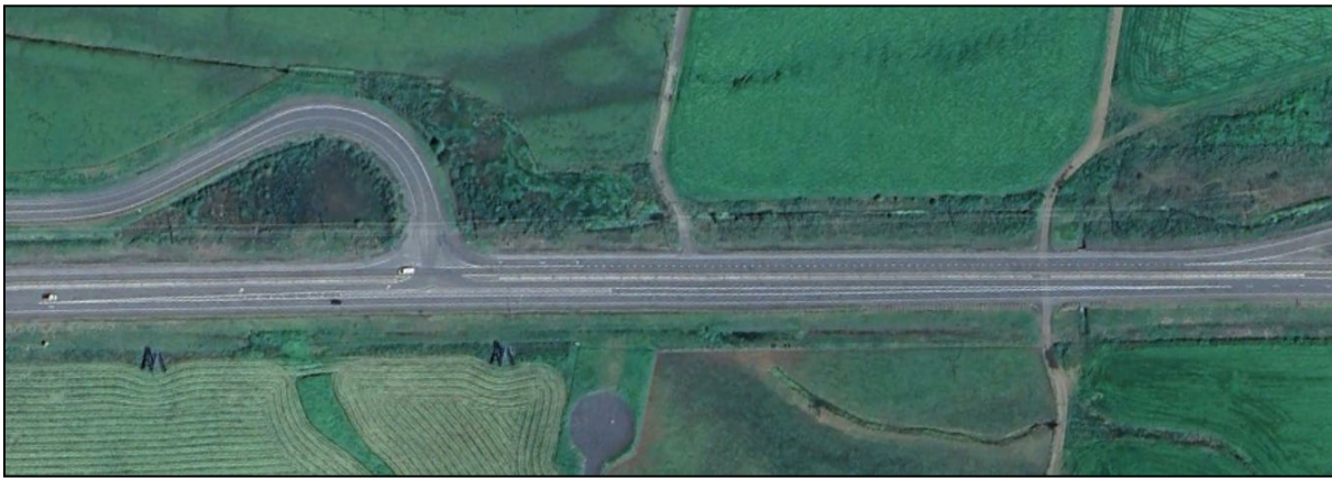
Figure 3-8. Unsignalized continuous green T intersection: OR 6 US east of Tillamook, Oregon.
