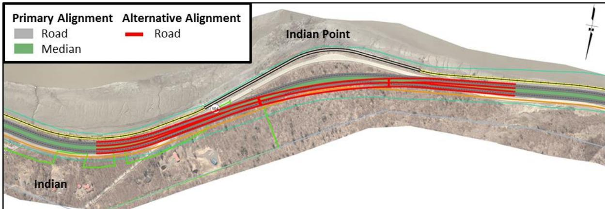
**Figure 14:** *Indian Point Tunnel Alignment Alternative*
