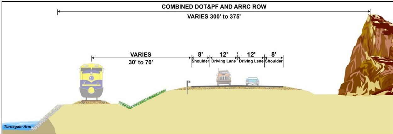
**Figure 2:** Simplified Existing Typical Section, Looking North
