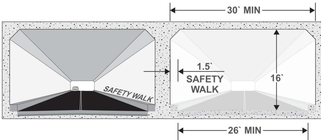
**Figure 12:** Minimum Tunnel Cross-Section
