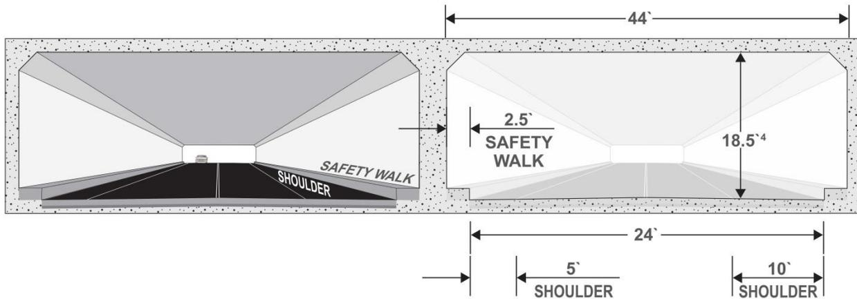
**Figure 13: Desirable Tunnel Cross-Section<sup>12</sup>**
