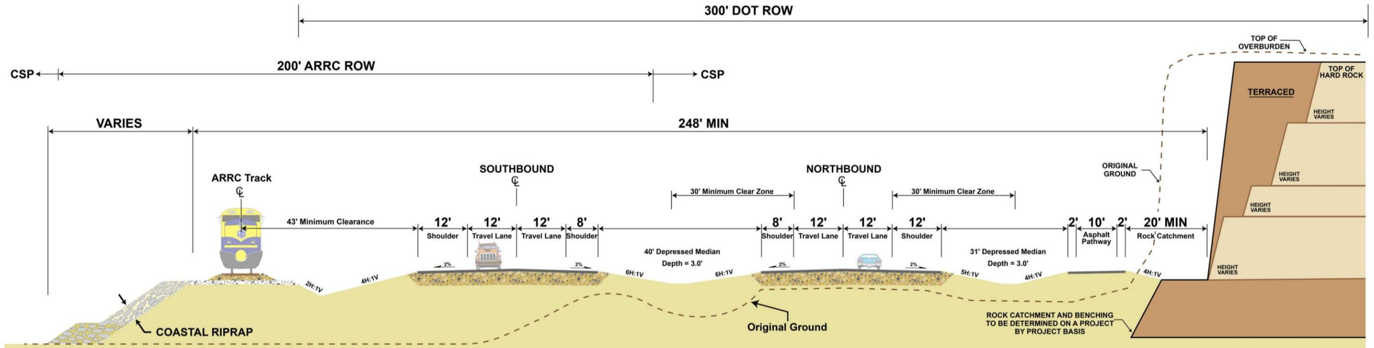
Figure 8: Proposed Four-Lane Divided Highway and Separated Pathway Concept
