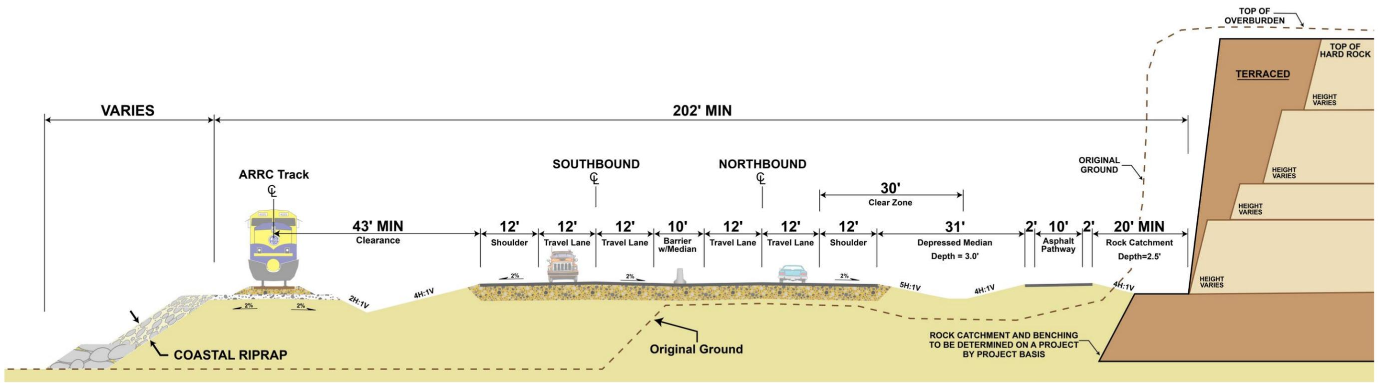
Figure 11: Barrier Median Cross-Section
