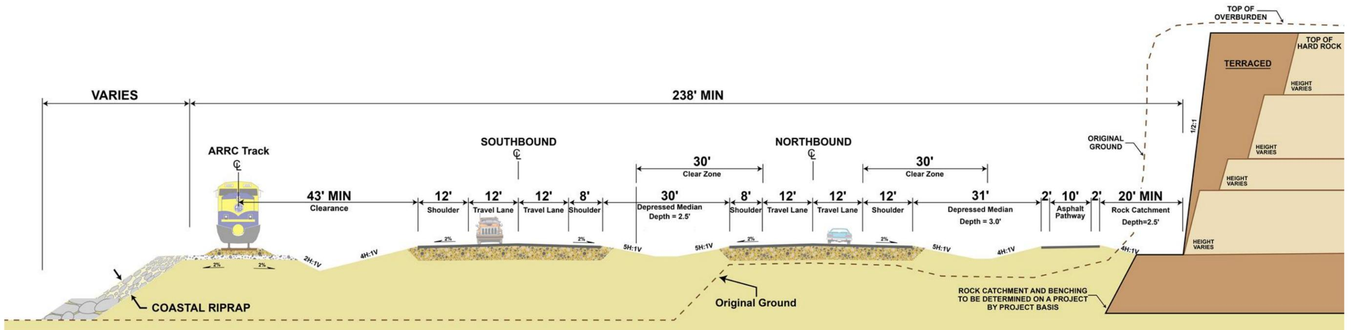
Figure 10: 30-foot Median Cross-Section, MP 111-114
